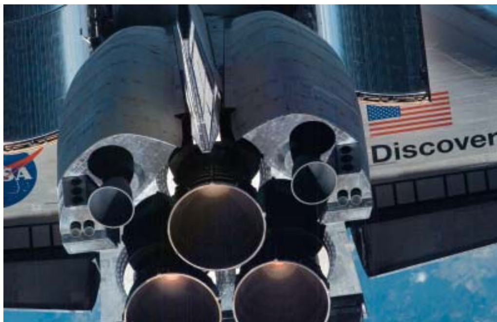
A close-up view of Discovery's tail section. Visible are the Shuttle's main engines, vertical stabilizer, orbital manoeuvring system (OMS) pods and a portion of the aft cargo bay and wings. NASA
