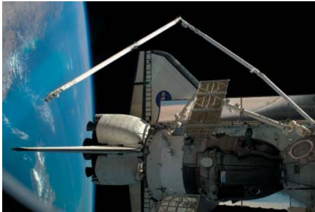
An unusual photograph showing both a Soyuz and Space Shuttle docked to the Space Station. Both the Shuttle's and Station's robotic arms are also visible. NASA
