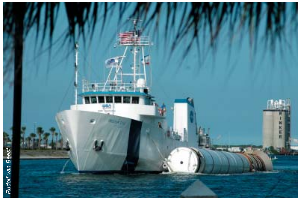
The Freedom Star with STS-118/Endeavour's left booster after retrieval from the ocean.
