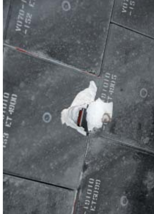
Photo of the troublesome gouge taken after Endeavour had returned to Earth. NASA
