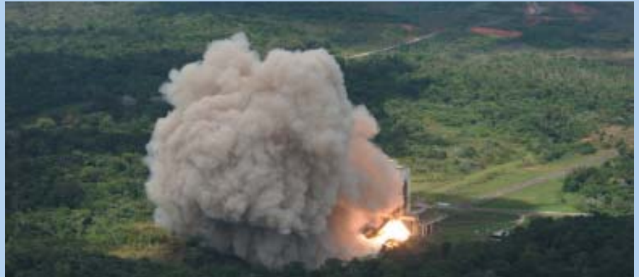
The P80 motor test firing.
